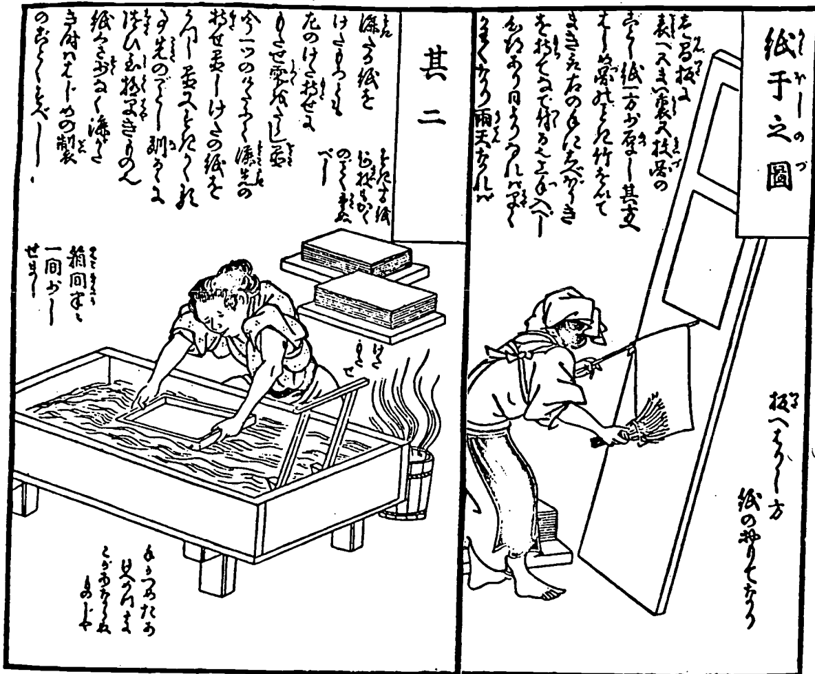
The vatman making a sheet of paper on the mould.
