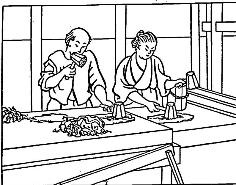
Beating kozo pulp with wooden hammers or mallets.
